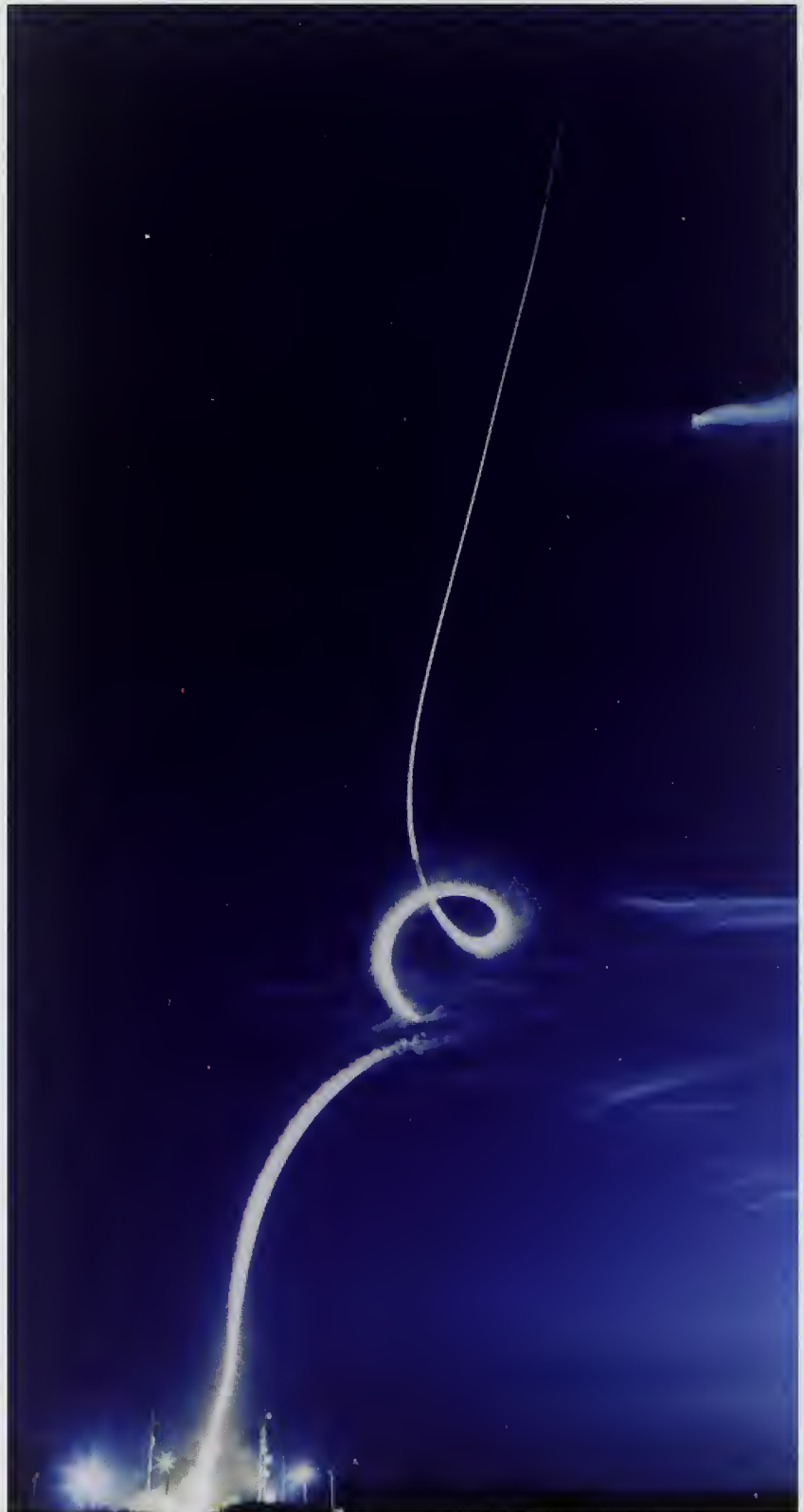
Fig. 5-15. The curly-cue in the Theater High Altitude Area Defense (THAAD) contrail is part of a purposeful maneuver to burn off excess fuel before the missile proceeds down range. The first THAAD intercept occurred during the tenth flight on 10 June 1999.
